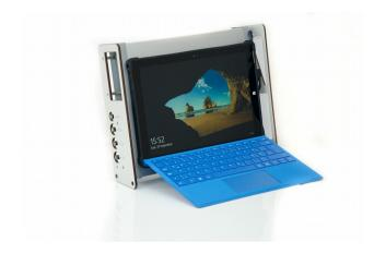
**4T2<sup>™</sup> Broadcast Multi Probe 3000** is a custom design to provide a cost effective, compact and robust, highly integrated measurement system for digital broadcasting (DVB-T/-T2) based on the latest generation tablet computer.
